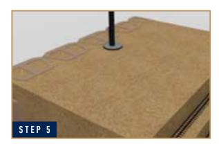
Insert fence post vertically into the TopGuide form and carefully fill with concrete
