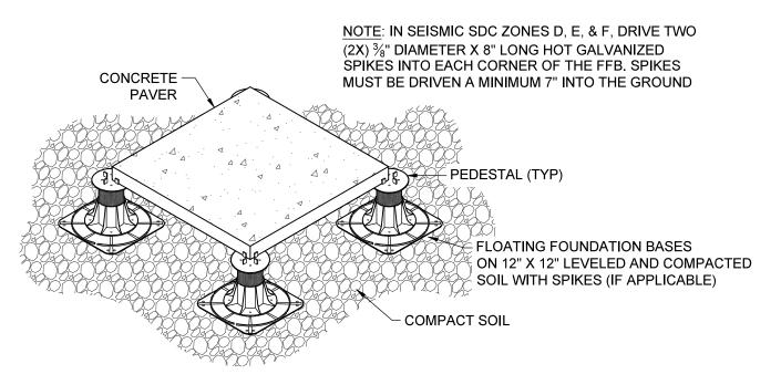
PEDESTALS ON FFBs (FLOATING FOUNDATION BASES)
