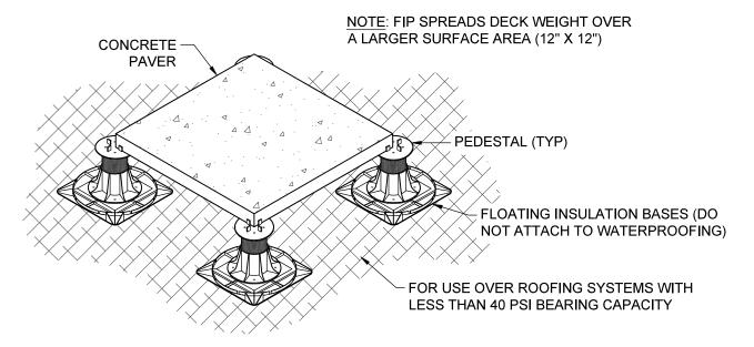
PEDESTALS ON FIBs (FLOATING INSULATION BASES)
