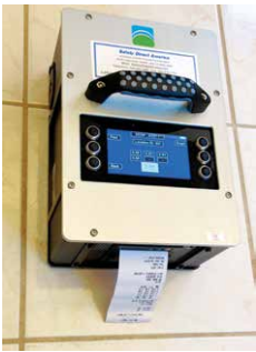
BOT-3000 Universal Walkway Tester Digital Tribometer Typical Belgard Paver DCOF wet values 0.6 to 0.75
