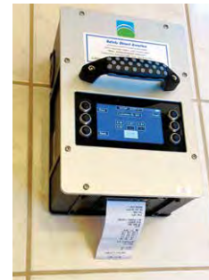
BOT-3000 Universal Walkway Tester Digital Tribometer
