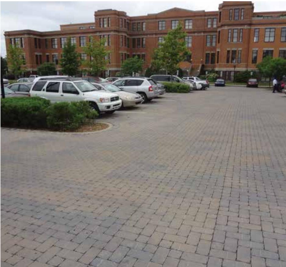
Permeable pavement solves the need for parking space, and the need for stormwater management.
