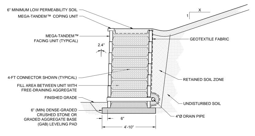
PLACE DENSE GRADED CRUSHED STONE OR GRADED AGGREGATE BASE (GAB) BETWEEN FACING UNITS BELOW THE FINISHED GRADE TO DAYLIGHT DRAIN PIPE THROUGH WALL FACE.
