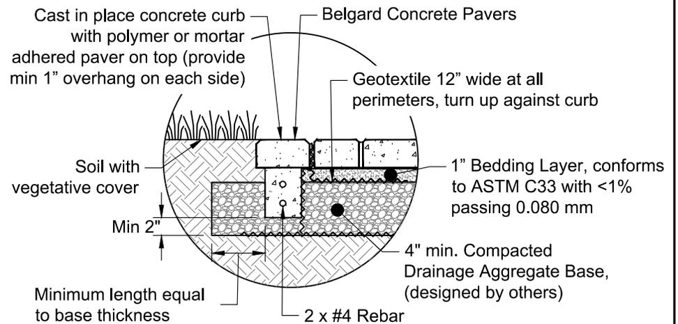
EDGE RESTRAINT - SAND SET ON AGGREGATE BASE
