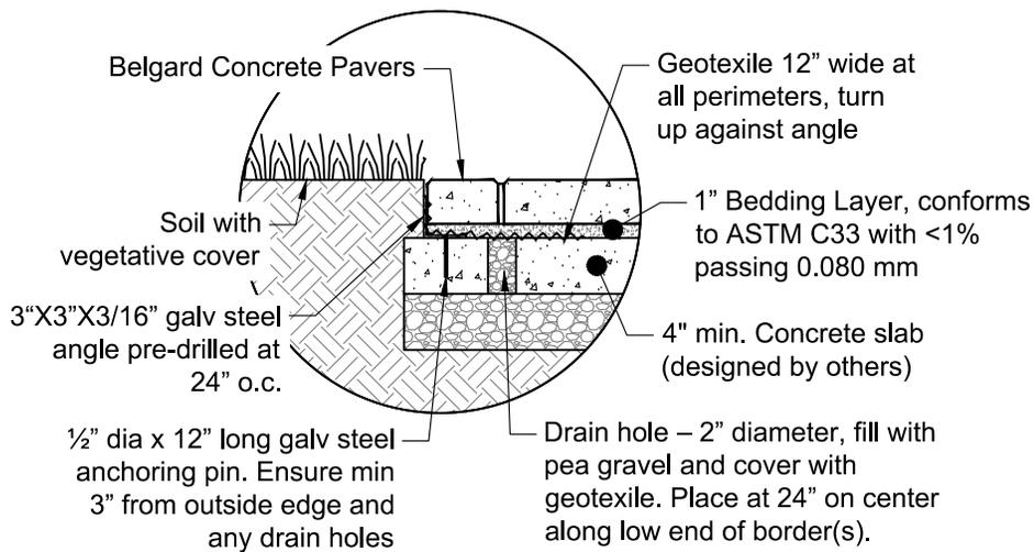
EDGE RESTRAINT - SAND SET ON CONCRETE BASE
